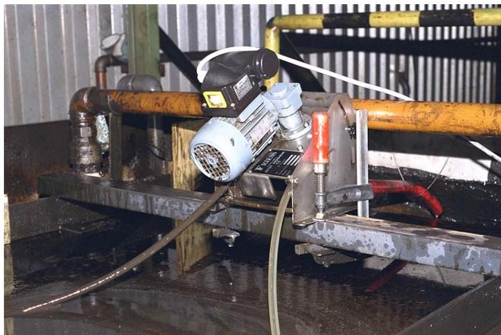
oil collector tube creates a movement on the water surface
